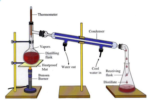
(Note: The above distillation apparatus is a common set up. This image has been adapted from <a href="http://oz.plymouth.edu/~wwf/distillation\_files/image001.jpg">http://oz.plymouth.edu/~wwf/distillation\_files/image001.jpg</a>)
