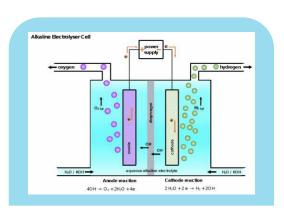
These electrolysers operate at temperatures between 100°–150°C and are often at elevated pressures of approximately 30 bar, the most energy efficient means of producing as well as for compressing the hydrogen gas. The electricity requirement to produce 1 kg of hydrogen range between 48 and 52kWh. Use of an alkaline electrolyte allows for the use of low-cost non-precious metal catalysts, such as nickel, for the electrodes, instead of more expensive platinum electrodes.
