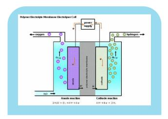
The electrons flow through the external circuit and the hydrogen ions selectively move across the PFM to the cathode.
